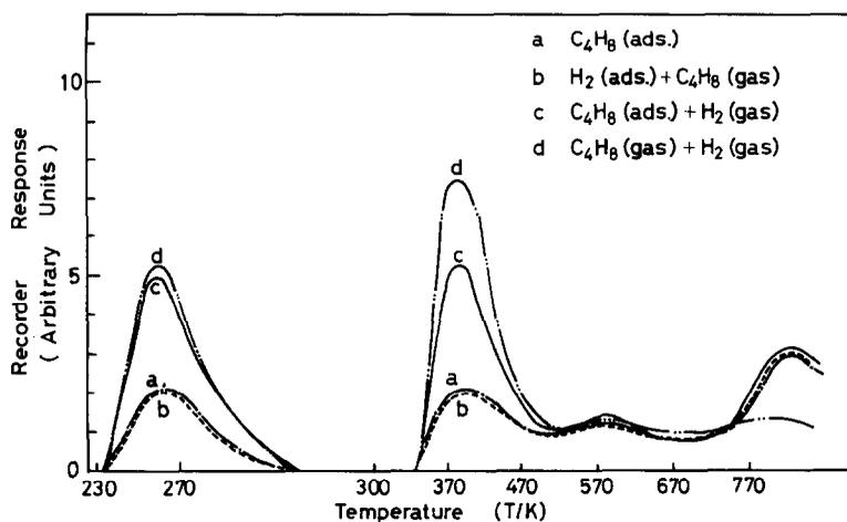
FIG. 1. TPD chromatograms of 1-butene on platinum. (a) 1-C<sub>4</sub>H<sub>8</sub> only was adsorbed. (b) H<sub>2</sub> was preadsorbed and 1-C<sub>4</sub>H<sub>8</sub> was subsequently admitted. (c) 1-C<sub>4</sub>H<sub>8</sub> was preadsorbed and H<sub>2</sub> was subsequently admitted. (d) 1-C<sub>4</sub>H<sub>8</sub> and H<sub>2</sub> were simultaneously admitted.
